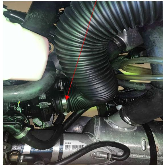
**10** Fasten the other side of the flexible hose to the air filter adaptor and mount the adapter to the hull
